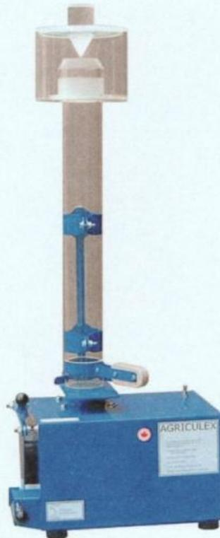
**This is a seed cleaner designed for precision cleaning of small samples of small-seeded crops. It can handle samples weighing up to about 10 grams.**
