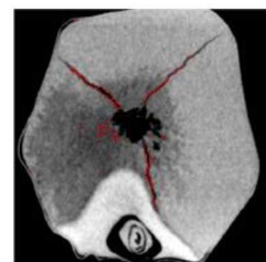
Quantification of cracks on a Corn seed
